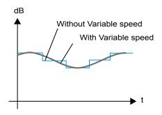
The AQUACIAT can be equipped as an option with a variable speed motor, enabling the fan to start gradually (all-season operation).
